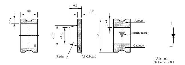
Electrodes: Au Plating Encapsulating Resin: Epoxy Resin Package: BT Resin
